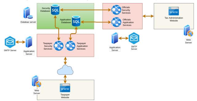
In the following conceptual architecture diagram, we can see how these components interact.
